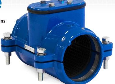
The Watertool Spade Valve is a cast iron valve, supplied with 2 aluminium support blocks, a manual guillotine-assembly and a stainless steel spade. After the valve is installed onto the pipe, the two aluminium support blocks are mounted onto the upper bolts of the valve unit after which the spade is pushed into the PE pipe wall by means of the guillotine. One of the characteristics of the patented invention is that the spade cuts into the PE pipe wall without completely cutting it.
