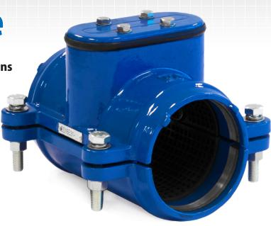
The Watertool Spade Valve is a cast iron valve, supplied with 2 aluminium support blocks, a manual guillotine-assembly and a stainless steel spade. After the valve is installed onto the pipe, the two aluminium support blocks are mounted onto the upper bolts of the valve unit after which the spade is pushed into the PE pipe wall by means of the guillotine. One of the characteristics of the patented invention is that the spade cuts into the PE pipe wall without completely cutting it.
